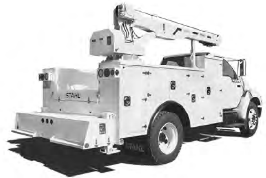
Shown with optional crane, bumper and manual outriggers.
