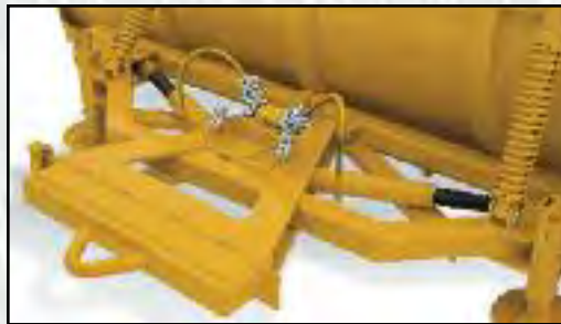
▲ Heavy-duty tubular push frame distributes plowing stresses.
